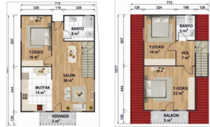
Zemin Kat Planı 74\text{m}^2 + 5\text{m}^2 \text{ VERANDA} = 79\text{m}^2 1. Kat Planı 50\text{m}^2 + 5\text{m}^2 \text{ BALKON} = 55\text{m}^2
