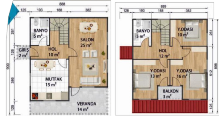
Zemin Kat Planı 55\text{m}^2 + 16\text{m}^2 \text{ VERANDA} = 71\text{m}^2 1. Kat Planı 56\text{m}^2 + 3\text{m}^2 \text{ BALKON} = 59\text{m}^2
